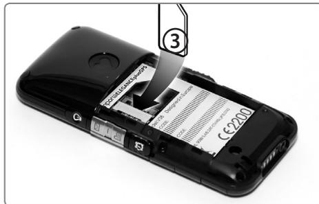
Insert the SIM card with the gold chip down and the clipped corner on the top left.
