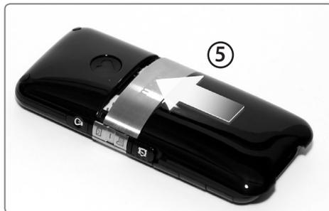
Slide the cover with light pressure until it snaps into place.
